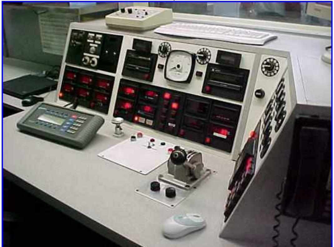
The readout at 9000 RPM and 505 to 510 horsepower was surpassed only by the muffled scream of the engine. Full throttle for up to six seconds is enough to make the exhaust headers glow red. The newer engines are tested with 98 octane fuel and can be hooked up to either the customers ECU or a Porsche calibrated engine control module. The recorded results are available to the customer.
